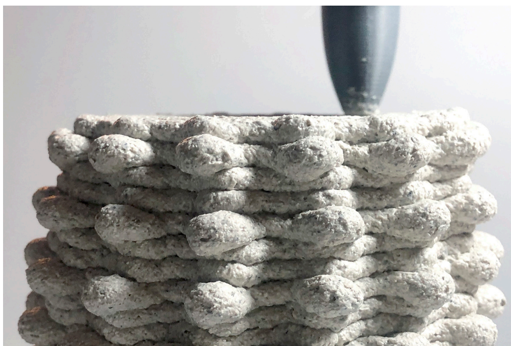
Figure 5. 3D printing waste material process. © bioMATTERS, LLC
