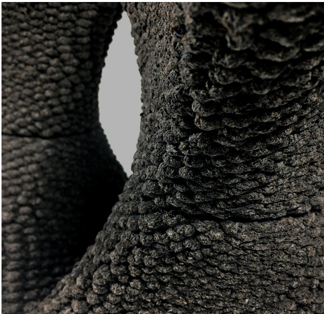
Figure 7. D printed waste material component detail. © bioMATTERS, LLC
