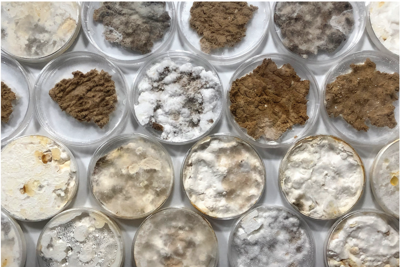
Figure 1. Waste material paste substrate with growing mycelium. © bioMATTERS, LLC
